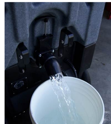
Drain water from Recovery Tank
