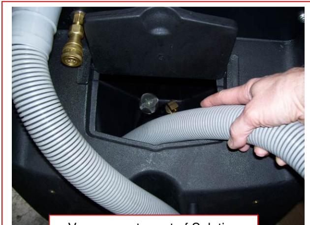
Vacuum water out of Solution Tank
