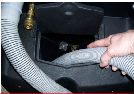
Vacuum acid solution out of Solution Tank
