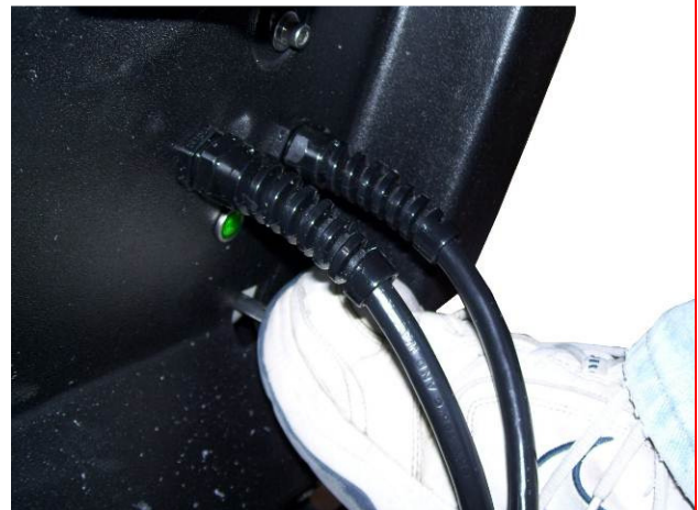
PRESSING THE PUMP PRIMING VALVE
